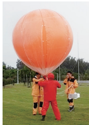
Releasing a balloon to calculate the wind speed profile
